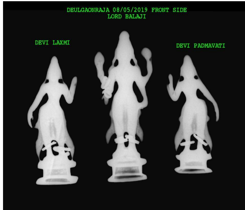
Figure 8. Computerised Radiography Inspection Image – Front Side
